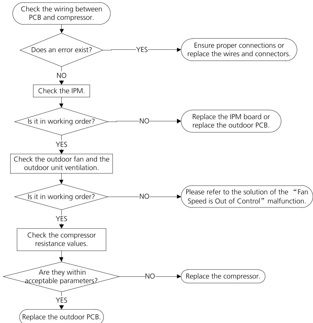
**Note:** For certain models, outdoor PCB could not be removed separately. In this case, the outdoor electric control box should be replaced as a whole.
